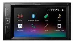
We have found that some stock of the Pioneer AVH and DMH series radios (DMH-A240BT, DMH-A340DAB etc) have been sold with old firmware that does not work with our 29 series steering wheel controls. Very early models of the SPH-DA160 were also affected.
